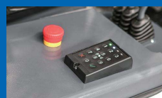
Emergency switch + Pin-code lock
